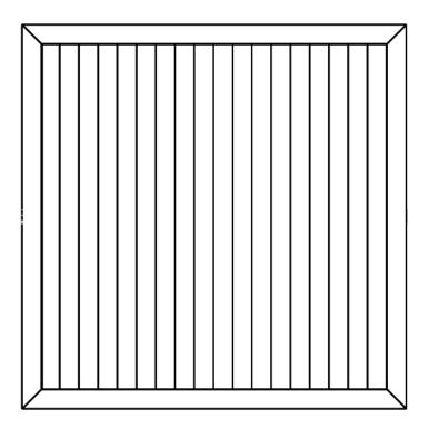
3. Place the top layer on top of the frame and beams and attach them with woodscrews 6x50 in the drilled holes.
