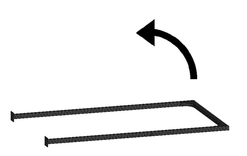
Assemble first section lying on the ground and then raise it.
