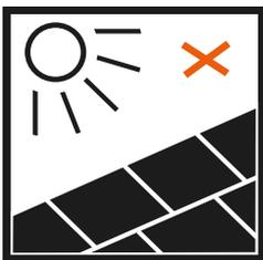
**11.** In areas that are exposed to intense or direct sunlight, the product must be protected during the conditioning, installation, and usage, by covering the light source. Exposure to excessive UV rays can result in fading, degradation, colour variation and crumbling. If you plan expose tiles/mats to direct sunlight ask for UV protection option.
