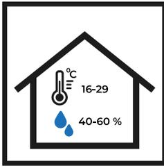
**1.** RUBTILER tiles and mats must be stored in an indoor, climate controlled space and be protected from fire, dirt, water and other elements. Temperature must be maintained between 16°C and 29°C with a relative humidity between 40% and 60%.
