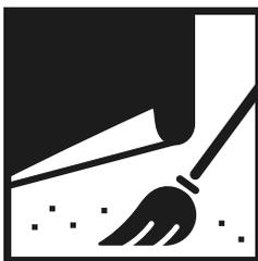
**5.** Substrates needs to be cleaned of dirt, dust, debris cause those could interfere the final surface. Moisture in the substrate negatively affects rubber tiles/mats and should be eliminated prior to installation.
