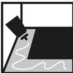
**6.** Tiles can be stuck to the substrates with double face tape or not caustic glue/adhesive (sometimes silicon glue is enough). Glue all tiles to the floor is not a necessity, it depends from particular need of installation and product shape. We recommend to glued down at least tiles/mats placed on edges of whole covered area.
