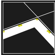
**10.** You can also use plastic pins for additional tiles connecting (but min thickness for pins is 25mm tile, there are 2 or 4 pin holes on only two sides of tiles and you connect them with plastic pins like 55 or 70 mm long). To some of our tiles/mats you can use Four Pin Plate Connector, while you can connect tiles on the corners (with one connector) from the bottom of the tiles.
