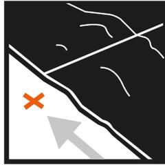
**8.** While installing, tiles/mats needs to be pushed up one to each other, but not extremely cause that can make bulges.
