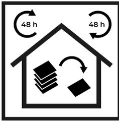
**2.** 48 hours prior to installation and 48h after, product must be site conditioned at wellventilated areas in temperature between 18°C and 26°C. We recommend to take tiles/mats out of pallet, separately, laid down for correct shape regaining and flatten out before installation.
