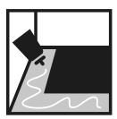
6. Tiles can be sticked to the substrates with double face tape or not caustic glue/adhesive (sometimes silicon glue is enough). Glue all tiles to the floor is not a necessity, it depends from particular need of installation and product shape. We recommend to glued down at least tiles/mats placed on edges of whole covered area.
