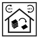
2. 48 hours prior to installation and 48h after, product must be site conditioned at wellventilated areas in temperature between 18°C and 26°C. We recommend to take tiles/mats out of pallet, separately, laid down for correct shape regaining and flatten out before installation.
