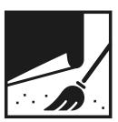
**5.** Substrates needs to be cleaned of dirt, dust, debris cause those could interfere the final surface. Moisture in the substrate negatively affects rubber tiles/mats and should be eliminated prior to installation.
