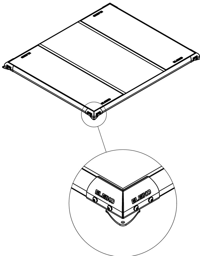
**Tighten frame and screws just to hold them in place.
