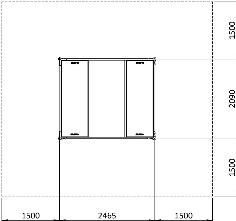
Add sufficient clearance, not less than 1,5 m, on all sides.
